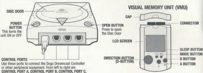
AND CONTROL PORT D. Use each port to connect controllers for players 1 to 4 respectively.
